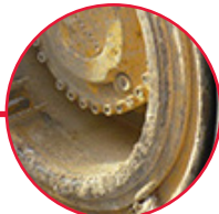
Poorly cleaned rim
