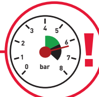
Network overpressure (over 6 bar)
