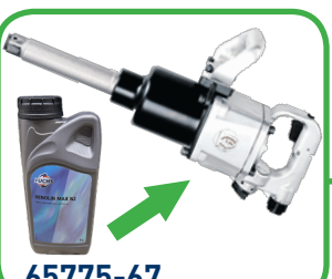
4-5 drops of special lubricant into the air inlet
